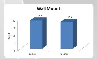
Integrated with an inverter "variable speed" compressor, SkyAir systems deliver the capacity required to maintain desired room conditions and reduce energy consumption with SEER levels up 18.6. This technology minimizes temperature fluctuations and provides continuous cooling and heating comfort with maximum energy savings.
